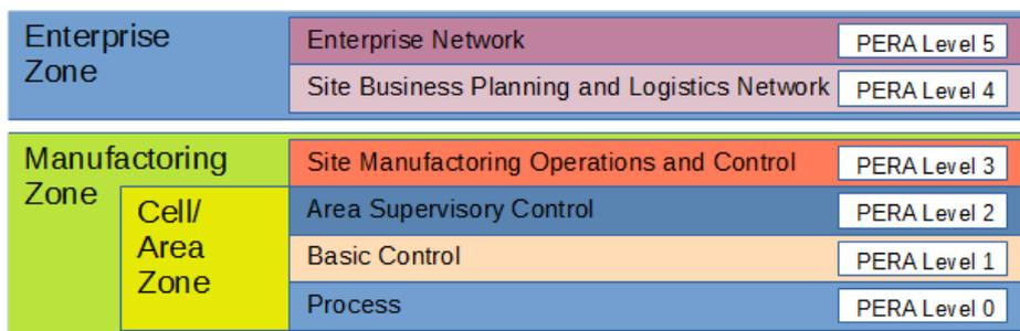
Fig. 1. Control Hierarchy of ICS according to [1]
